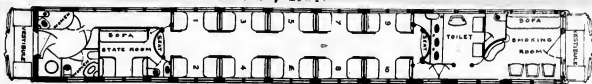
FLOOR PLAN OF CANADIAN NORTHERN SLEEPING CAR. Sleeping Car, Canadian Northern Ry.
